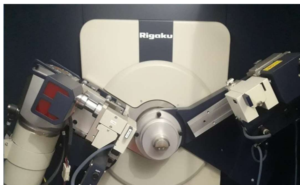
Fig6:X-ray powder Diffractometer under DST-FIST project of Department
