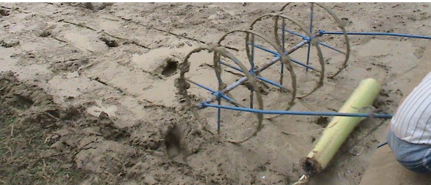
Cross marking in single operation with the innovative Portable SRI Marker
